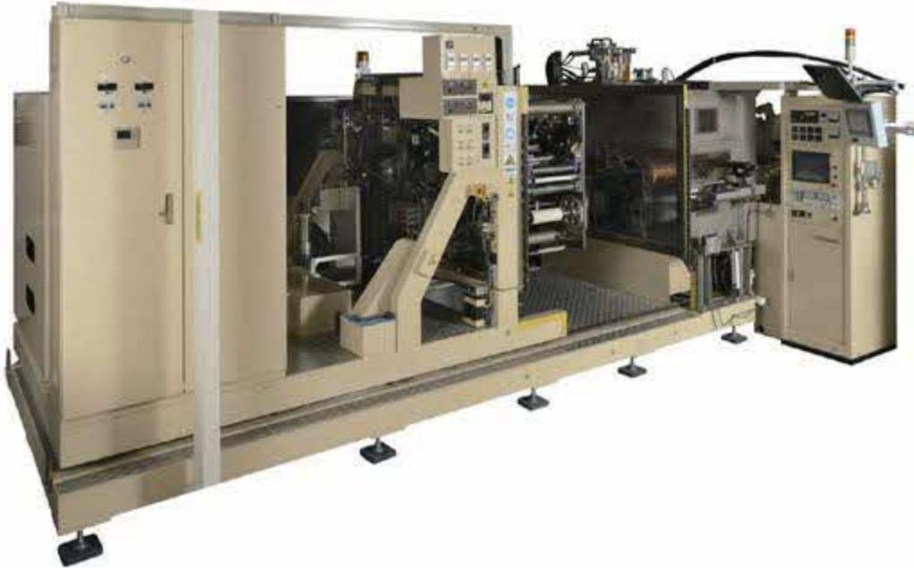
This vacuum deposition device makes it possible to manufacture film capacitor electrodes, lithium battery electrodes and the like by roll to roll. The evaporation sources that can be mounted are resistance heating crucibles, radiant heating crucibles, and E/B sources. A plasma source is also available to improve adhesion between the base material and the deposition layer. It is also capable of handling double-sided deposition.
